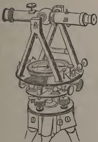
Surveyor's or Engineer's Transit Instrument.
